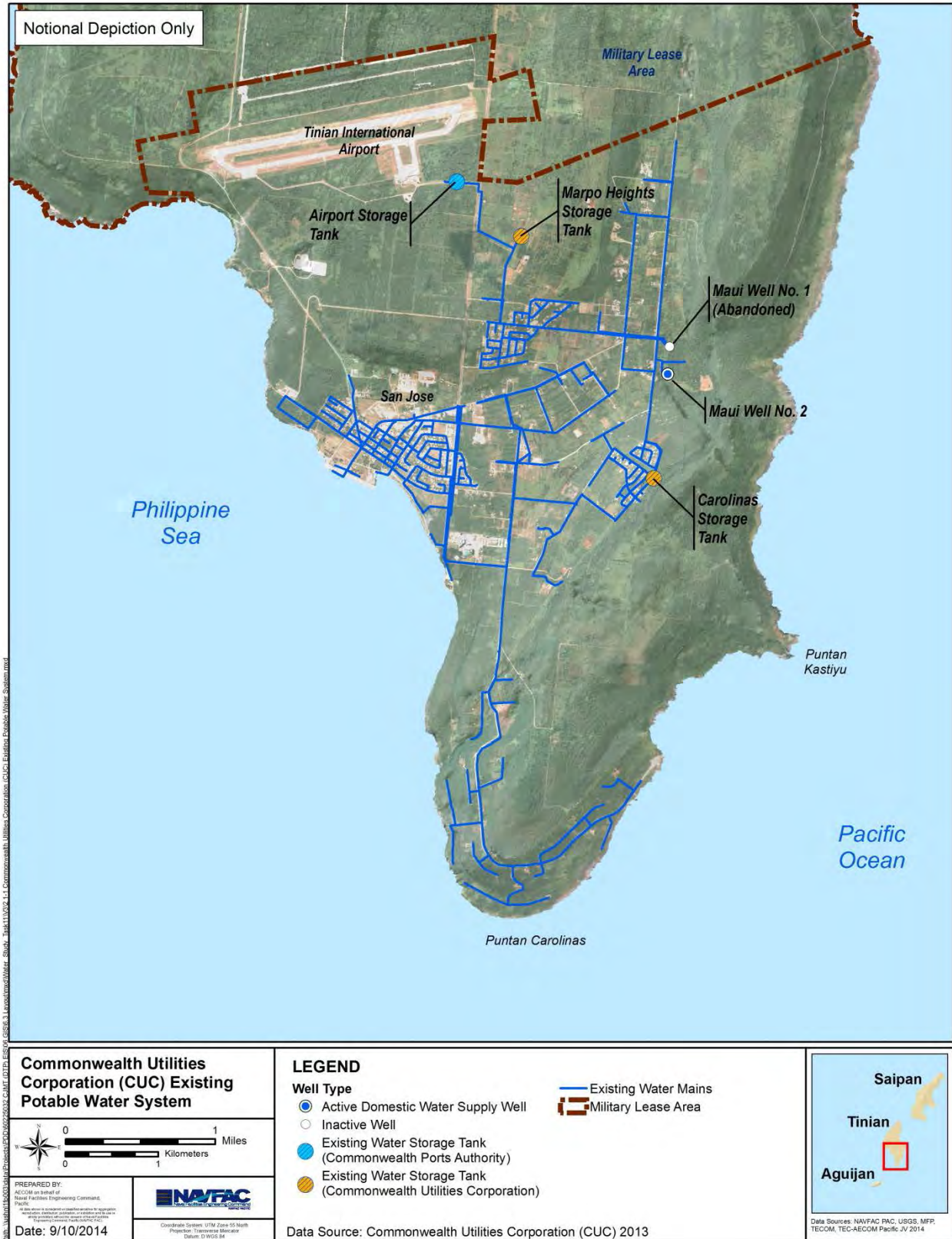
Figure 2.1-1. Commonwealth Utilities Corporation (CUC) Existing Potable Water System
